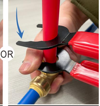
The faceplate with size markings must be faced down and use only this faceplate to disconnect the tubing
