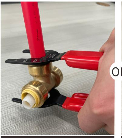
Open the clamp fork little wider and position like this to remove the tubing
